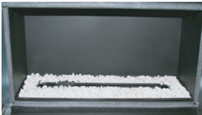
Figure 39 - Filling the tray with media
